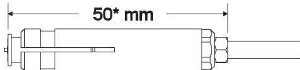
Fig. 4: Set-up of the chuck for gun ESP 1 K for studs with max. length 40 mm
