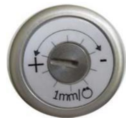
Figure 3: setting disk of the pistol ESP 1 S
