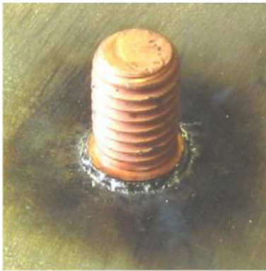
Fig. 7: Weld with energy supply correctly set and an even ring of splashes
