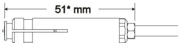
Fig. 2: Set-up of the chuck for gun ESP 1 S for studs with max. length 40 mm
