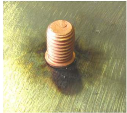
Fig. 9: Weld with energy set too low, consequently no visible ring of splashes present
